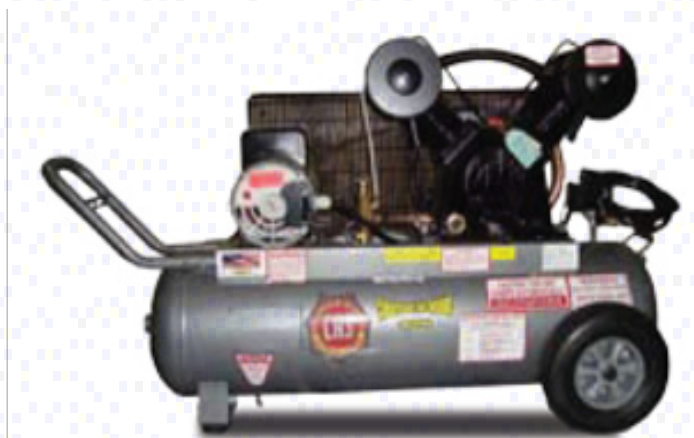
Typical Portable Air Receiver with Mounted Compressor
